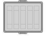
The AK2 modular system can cover a wide range of applications, as it offers the right solution for all installation tasks. The modular system consists of a basic box, a front part and attachment accessories in numerous variants. This allows individually configured boxes to be assembled for pluggable electrical installation.
