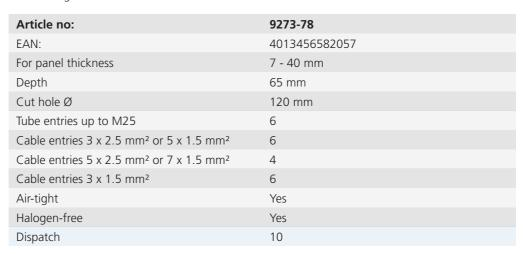
Air-tight  $\emptyset$  120 mm junction box with ECON® technology for an energy-efficient electrical installation in accordance with GEG. Extremely easy fitting thanks to toolless cable and conduit entry. The sealing membranes guarantee permanent air-tightness and at the same time retention of the cable or conduit. The large box volume provides plenty of installation space for various cable connections.
